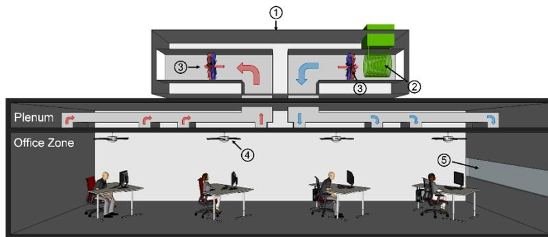
Figure 2. HVAC layout: (1) Rooftop air handling unit; (2) Heat pump and heat exchanger; (3) Fans; (4) Ceiling fan; (5) Window
