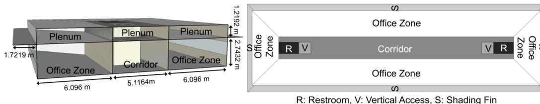
Figure 1. Building simulation model section cut (one floor) and simulation zones
