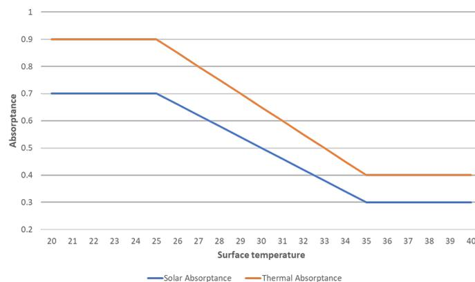
Figure 2. Optical (solar absorbance) and thermal (thermal absorbance) performance of the TC coating as the function of surface temperature.
