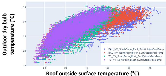
Figure 5. (a) Roof outside surface temperature of BAU and TC case concerning dry bulb temperature in SS scenario; (b) Roof outside surface temperature of BAU and TC case concerning dry bulb temperature in AS scenario; (C) Roof outside surface temperature of BAU and TC case concerning dry bulb temperature in NV scenario.
