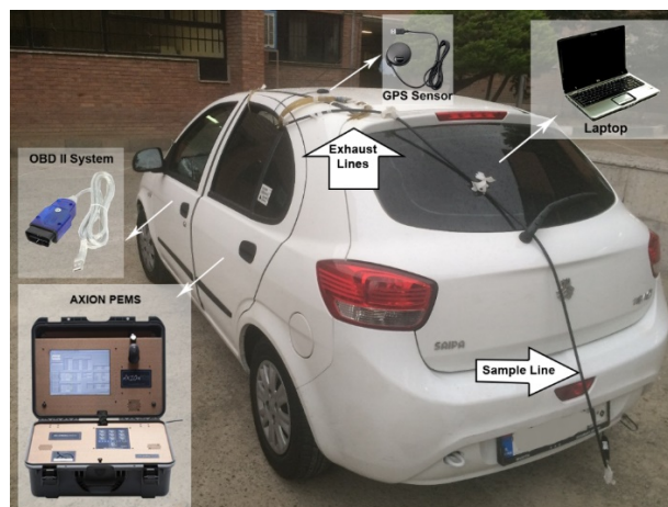
Figure 1. Installation of PEMS main components on the test vehicle
